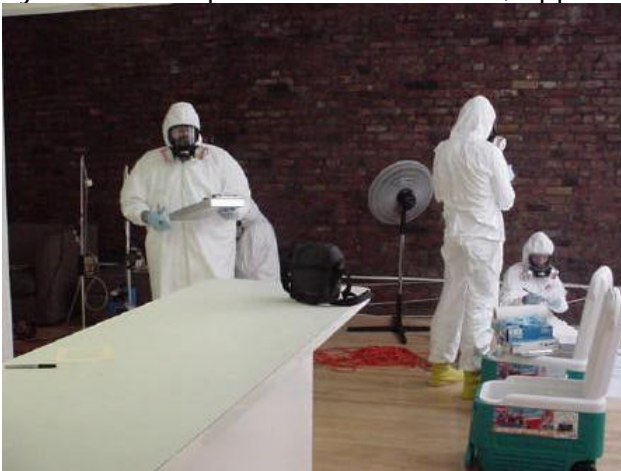
Figure 11: Post Clean Up Sampling – Note the protective attire of the workers and compare to previous photos – Photo: EPA Confirmation Cleaning Study 110 Liberty Street
